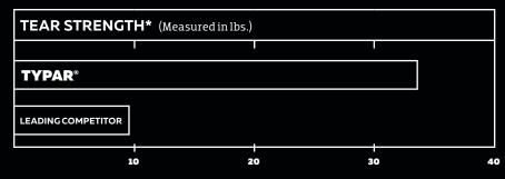
$^{\star}$ Based on published results for tear strength according to ASTM D5733-99 testing.
