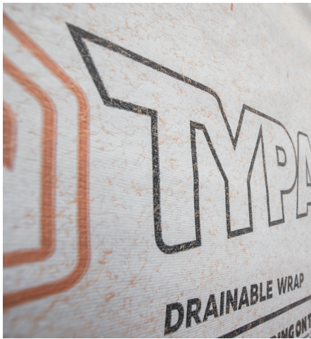
Figure 1. Randomly-oriented orange polypropylene fibers on TYPAR DrainableWrap and TYPAR DrainableWrap Commercial.
