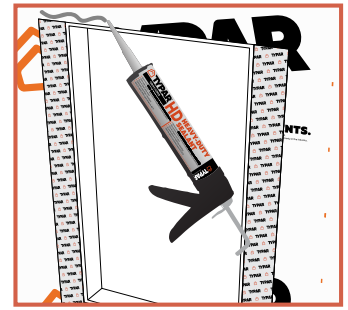
Sealant Applied to Head Flange
