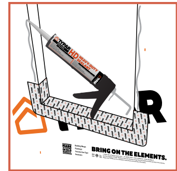
TYPAR HD Sealant Applied Around Window Perimeter
