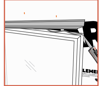
Drip Cap Set Onto Head Flange
